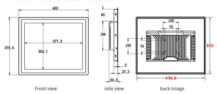
Warm reminder: The size unit is millimeter (mm), and the error is within  $\pm 0.5$ mm
