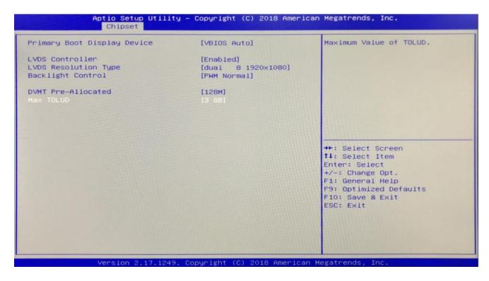
Primary Boot Display Device: Primary display boot (VBIOS Auto is automatically recognized, can also be set to VGA / HDMI
