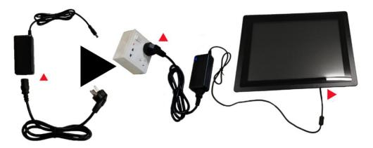
1. If the machine is not set to power on, press the "POWER" key switch after connecting the power supply.
