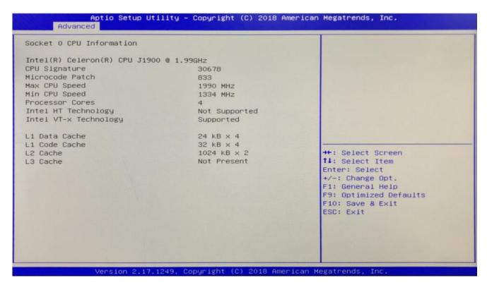
The read-only item contains the detailed information of the CPU, including the CPU manufacturer, model, frequency, cache size, etc.
