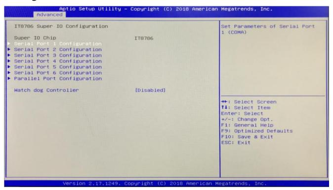
Contains serial port COM1~COM6 and parallel port (LPT port) configuration information and settings
