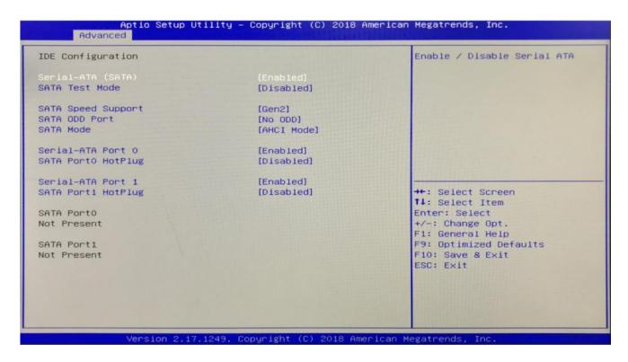
SATA Test Mode: Hard drive test mode
